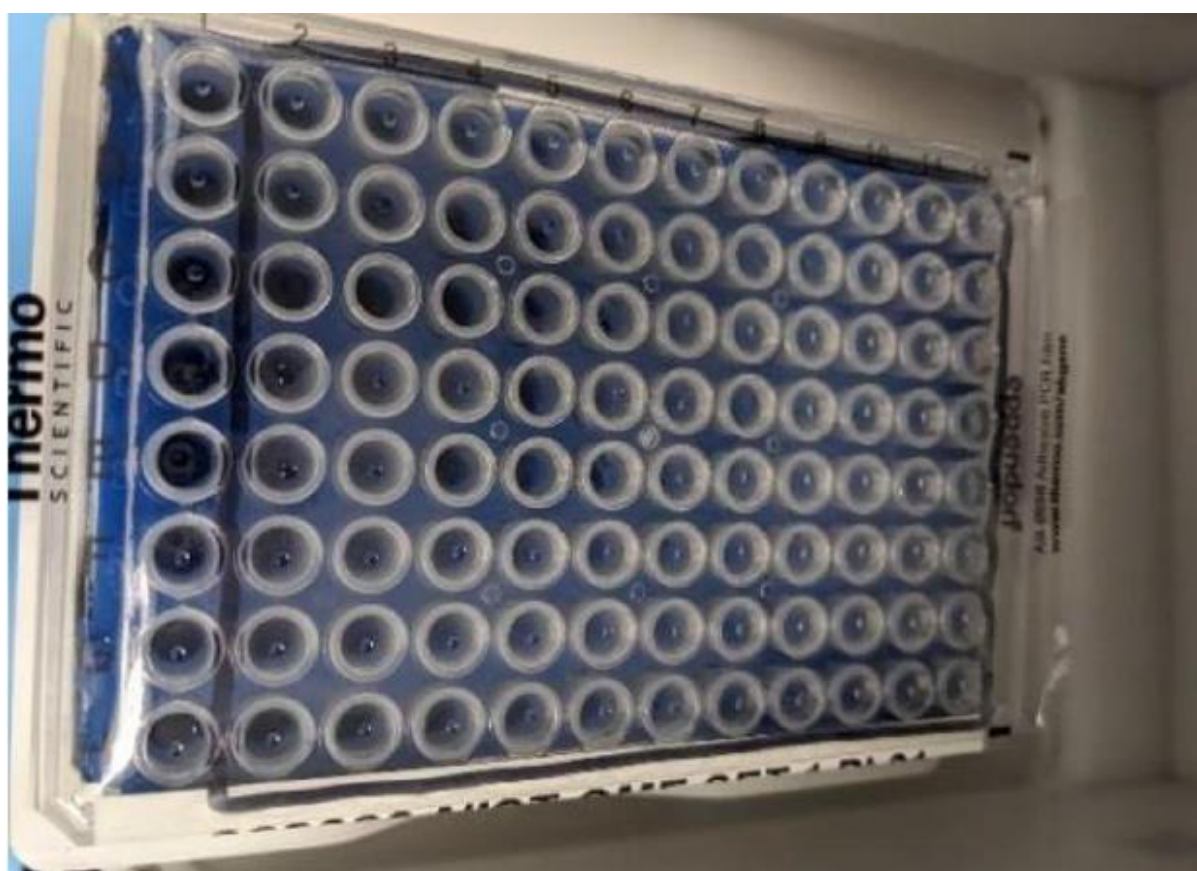
Figure 5 Example of a typical well aligned plate.
